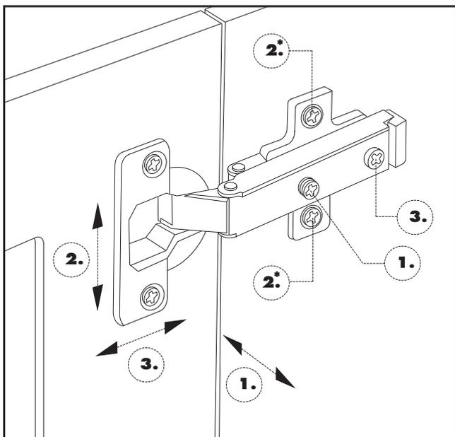
If the cabinet's doors appear out of alignment, this condition can be corrected with minor adjustment to the European hinges on each door.
